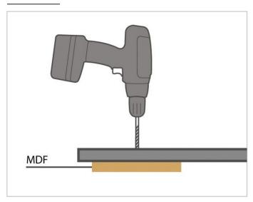
When drilling through the countertop completely, a sacrificial piece of MDF should be used on the underside of the hole to prevent flaking. For holes that do not need to go through the countertop completely, it is recommended a maximum hole depth of approximately 3/16in (8mm).
