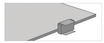
Solid 12mm FENIX NTM® countertops do not require any kind of edging strips. To finish edges, simply sand with a 240-grit sandpaper to soften the edge and then finish using Scotch-Brite™ with hard backer being careful not to sand the surface of the countertop. It is recommended that a small amount of linseed oil is applied to cut edges to achieve a smooth finish.
