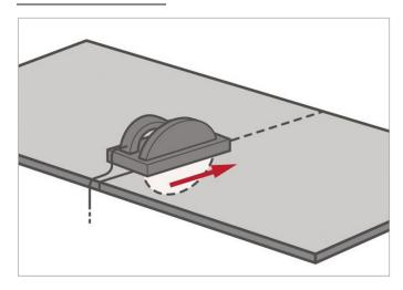
Note: Joint edges and final finished ends will require trimming to size when finished- please allow an additional 2-3mm for this.
