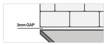
If you'd like to fit tiles above your Solid FENIX NTM® countertop, a small gap of at least 1/8in (3mm) is advisable to allow for the natural expansion of the work surface. Color matched 100% Silicone caulk must be used. This can also be done to any other wall surface.
