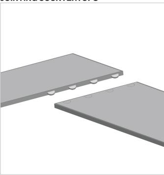
A clear 2-part epoxy resin is needed to bond two countertops together and will also work as a waterproof sealant. Follow the instructions carefully to ensure the correct ratio of hardener to adhesive is used.
