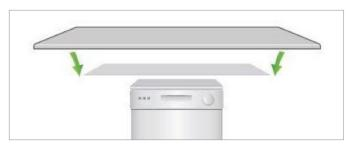
When installing a dishwasher or washing machine, ensure a protective moisture barrier is fitted correctly to the underside of your countertop.
