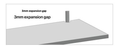
If holes need to be cut through the countertop, a space of at least 1/8in (3mm) should be included around the pipe to ensure there is room for the surface to expand and contrast. 100% silicone sealant must be used to fill this gap.
