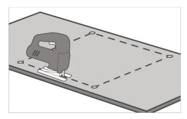
When cutting-out for sinks or other inset items, double check measurements or use a jig template- ensuring that it is clamped into position to avoid movement. Sharp cutting tools are required to ensure neat cuts. It is also important to support the countertop while cutting.
